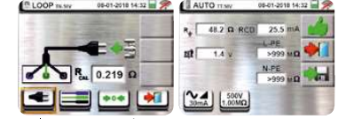
Zero-loop: compensation of the resistance of the test cables used for Loop impedance measurement.
