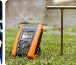
Measurement of earth impedance by voltammetric method.
