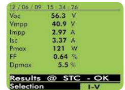
Detail of the single results of I-V Curve: OK
