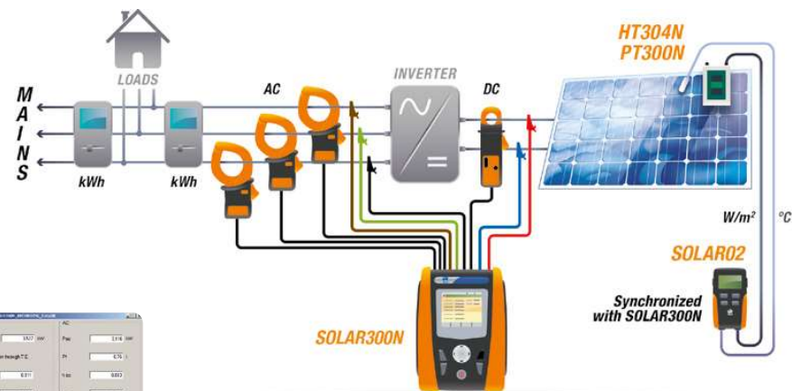
Connection diagram (three-phase system)
