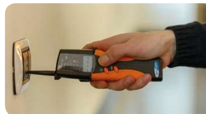
Phase detection function through conductive button.
